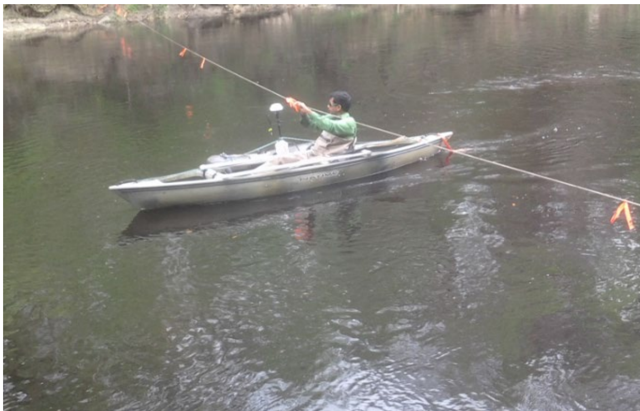
Figure 3. Moving boat discharge measurements.
