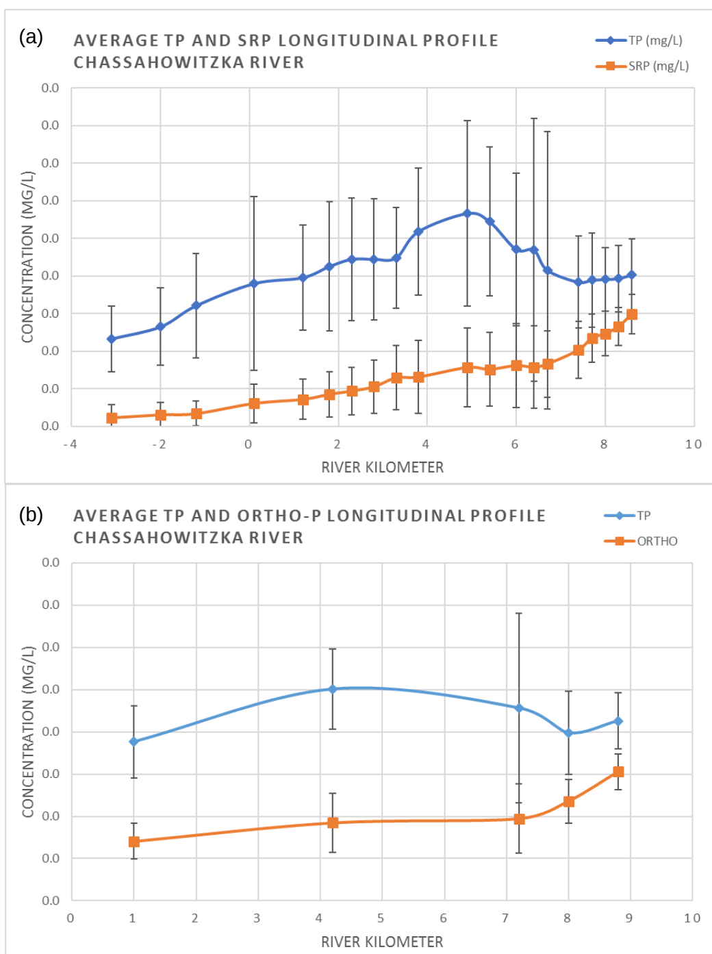
Figure 3-13 Longitudinal profiles of total phosphorous (TP) and soluble reactive phosphorous (SRP) concentrations from (a) the University of Florida 5 Rivers Project transect data collection effort between 1998 and 2011, and longitudinal profiles of total phosphorous (TP) and orthophosphorous (ORTHO) from the Coastal Rivers Project (P108) active water quality sampling network between 2006 and 2017. Error bars represent the standard deviation for each station.
