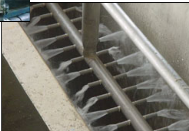
(Right) Rictor-type Air dispersion headers and nozzles
